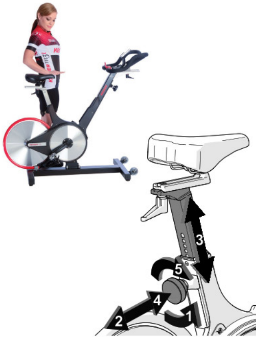
Figure 10. Seat Height Adjustment
